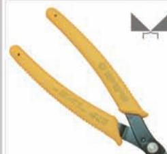
**TR 25 L:** Tool for a flush cut. Same characteristics as TR 25, but specially designed with longer handles to reduce the force needed by the operator. Safety clip for holding wire scraps securely after cutting available. Steel thickness 2.5mm. Tool length 160mm. ESD-safe handles version available
