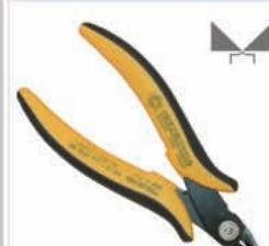
**TRE 03 NB:** Tool for a flush cut. Purposely designed as the simplified version of the TR 25 but with the same main characteristics. Safety clip for holding wire scraps securely after cutting available. Steel thickness 2.5mm. Tool length 138mm. ESD-safe handles version available
