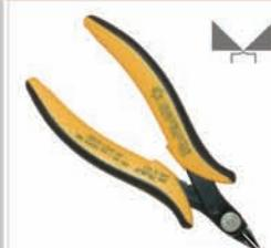
**TR 25 P:** Tool for a flush cut. With very sharp cutting edges, it is ideal for very delicate work in electronics, allowing access to difficult to reach areas. Safety clip for holding wire scraps securely after cutting available. Steel thickness 2.5mm. Tool length 132mm. ESD-safe handles version available
