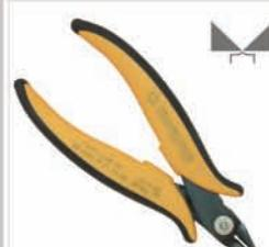
**TR 25:** Tool for a flush cut. One of the most popular cutting tool. Safety clip for holding wire scraps securely after cutting available. Steel thickness 2.5mm. Tool length 138mm. ESD-safe handles version available
