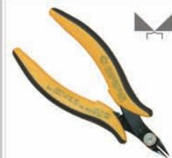
**TR 20 SM:** Tool for a flush cut. The reduced head's dimension and its pointed shape, allow access to difficult to reach areas. Similar to TR 20 M but with rounded edges. Safety clip for holding wire scraps securely after cutting available. Steel thickness 2.0mm. Tool length 132mm. ESD-safe handles version available.
