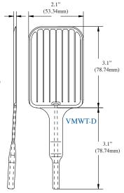
The PEEK® material selected for our molded wafer tips is an industry standard. They have excellent resistance to most chemicals. The nonsloughing carbon renders the wafer tips ESD safe. Excellent for applications up to 212°F (100°C).
