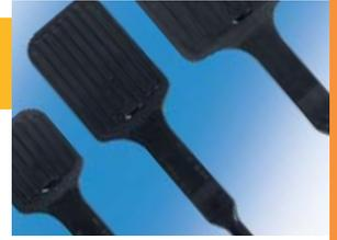
The PEEK® material selected for our molded wafer tips is an industry standard. They have excellent resistance to most chemicals. The non-sloughing carbon renders the wafer tips ESD safe. Excellent for applications up to 212°F (100°C).
