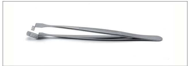
3WFG.SA Serrated handles. Tips: handling 2", top fingers, stepped bottom paddle with grid. OAL: 125mm
